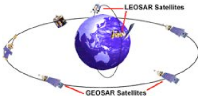
The COSPAS/SARSAT geostationary and polar orbiting constellations. Courtesy of www.cospas-sarsat.org
